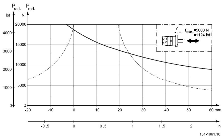
The output shaft runs in tapered roller bearings that permit high axial and radial forces. The permissible radial load on the shaft is shown for an axial load of 0 N as a function of the distance from the mounting flange to the point of load application.
