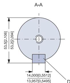
B: Cylindrical 2.25 in shaft for OMV with standard mounting flange
