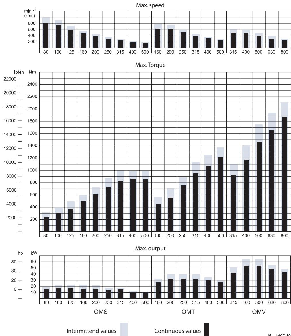
The bar diagrams above are useful for a quick selection of relevant motor size for the application. The final motor size can be determined by using the function diagram for each motor size.
