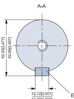
C: Cylindrical 2.25 in shaft for OMV with mounting flange SAE-C
