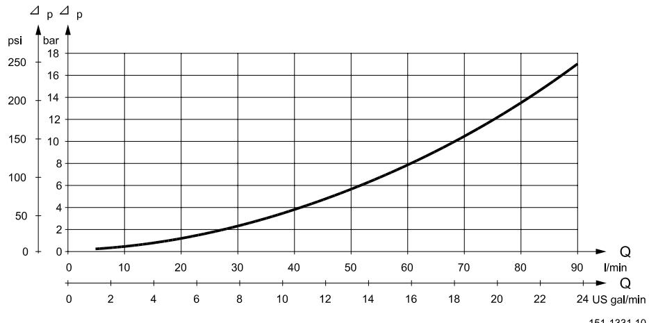
The curve applies to an unloaded motor shaft and an oil viscosity of 35 mm<sup>2</sup>/s [165 SUS]
