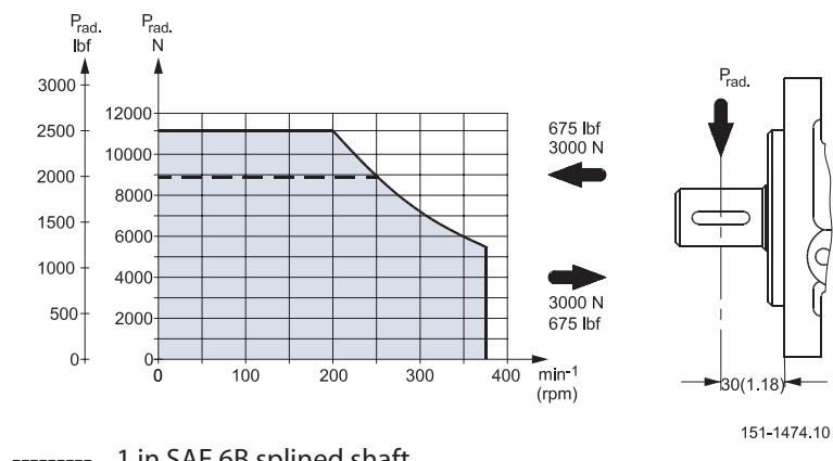
The drawing shows the permissible radial load when  $l = 30 \text{ mm}$  [1.18 in].
