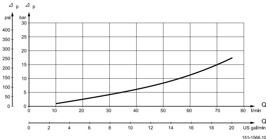
The curve applies to an unloaded motor shaft and an oil viscosity of 35 mm<sup>2</sup>/s [165 SUS]
