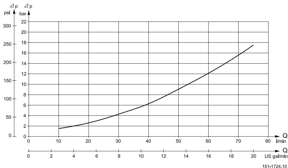
The curve applies to an unloaded motor shaft and an oil viscosity of 35 mm<sup>2</sup>/s [165 SUS]
