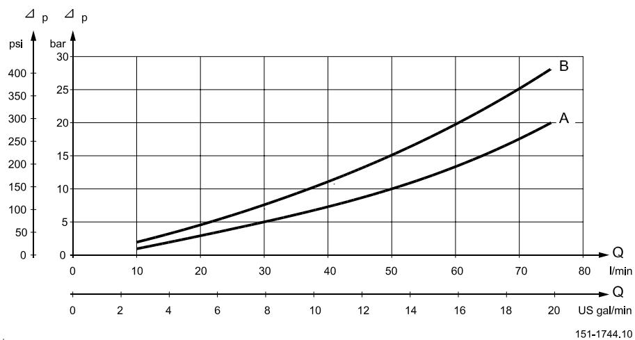
The curve applies to an unloaded motor shaft and an oil viscosity of 35 mm<sup>2</sup>/s [165 SUS]
